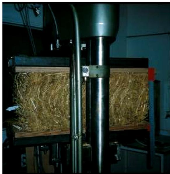
Fig. 4. Straw bale in compression test.
