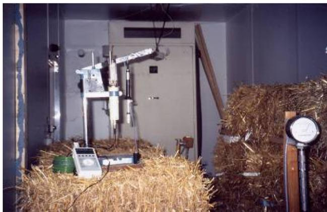
Fig. 3. Bales inside the climate chamber under compensation test condition.
